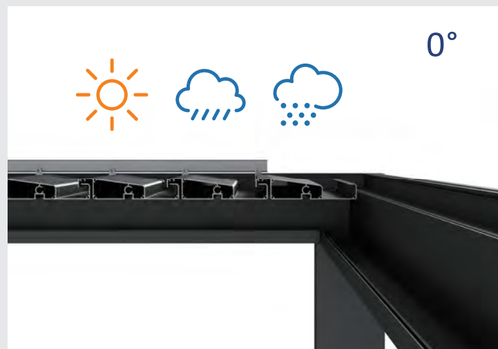
Louvers are designed such they will interlock to keep out the water, hot sun and snow. Deep channels in each louvers carry water away to the in-built surrounding gutter.
